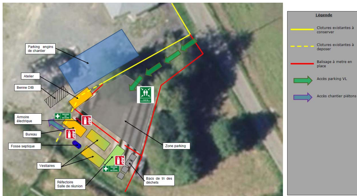
Figure 4 : Installation de la base vie Valgo
